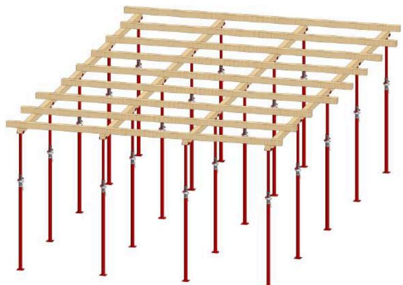
As inner pipes with U cap holding bearing beams of flooring grids can freely rotate with 360 degrees within outer pipe, this system allows grid directions to be adjusted in desired direction and to create local grid directions in different direction under the same flooring formwork.
