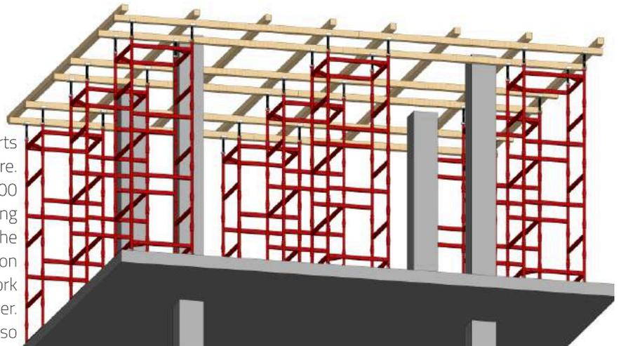
Precise height adjustment can be made with its adjusting elements with adjustable height available both under and over cartridge scaffolding towers. High quality concrete surfaces can be achieved with the formwork elements having even surface.
