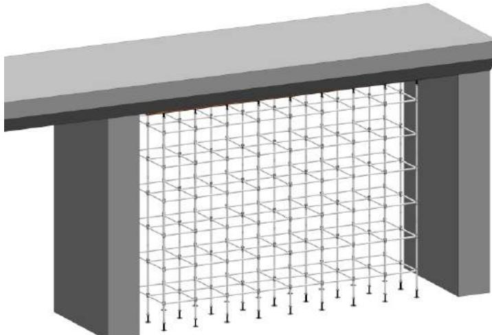
With the capability of 4 horizontal connections from each direction in the same nodal point to a post, this system can be used as a load scaffold for providing support to flooring molds and in facade works and industrial facility maintenance and repair works. That different functional systems are formed with standard elements makes this scaffolding system to be more preferable.
